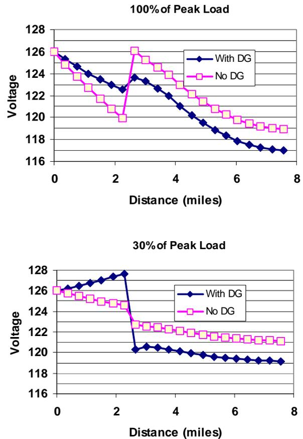
**Figure 4-7: Interaction of reverse power flow with regulator LDC. 100% DG penetration, DG lumped immediately downstream of regulator.**
