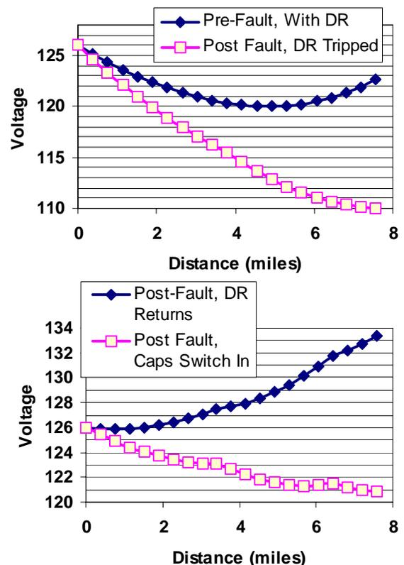
**Figure 4-10: Extremes of voltage caused by DG tripping due to a fault. Penetration 100%, load at 100% of peak. Order of events: pre-fault, DG trips, caps switch in, then DG returns.**
