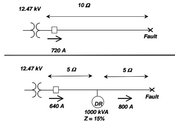
**Figure 4-1: Illustration of how DG can de-sensitize feeder protection**
