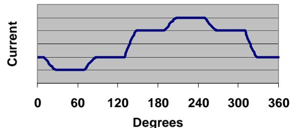
**Figure 3-12: 6-pulse load-commutated converter phase current (after isolation transformer)**
