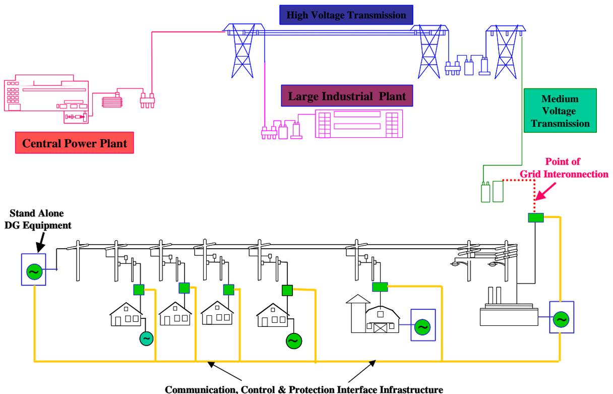
Figure 6-1: Conceptual scheme of a microgrid.
