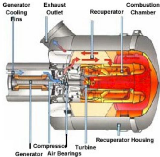
**Figure 3-2: Cutaway of a microturbine**
