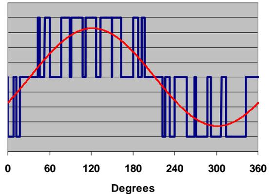
**Figure 3-14: Phase-phase voltage generated internally in a 3-phase VSI. Sinusoid is 60 Hz component of voltage created by PWM pattern.**
