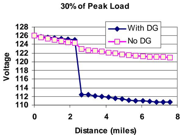
**Figure 4-8: Voltage profile for voltage regulator control made unstable due to triggering of reverse power flow feature, due to DG export flow. Penetration 25%.**
