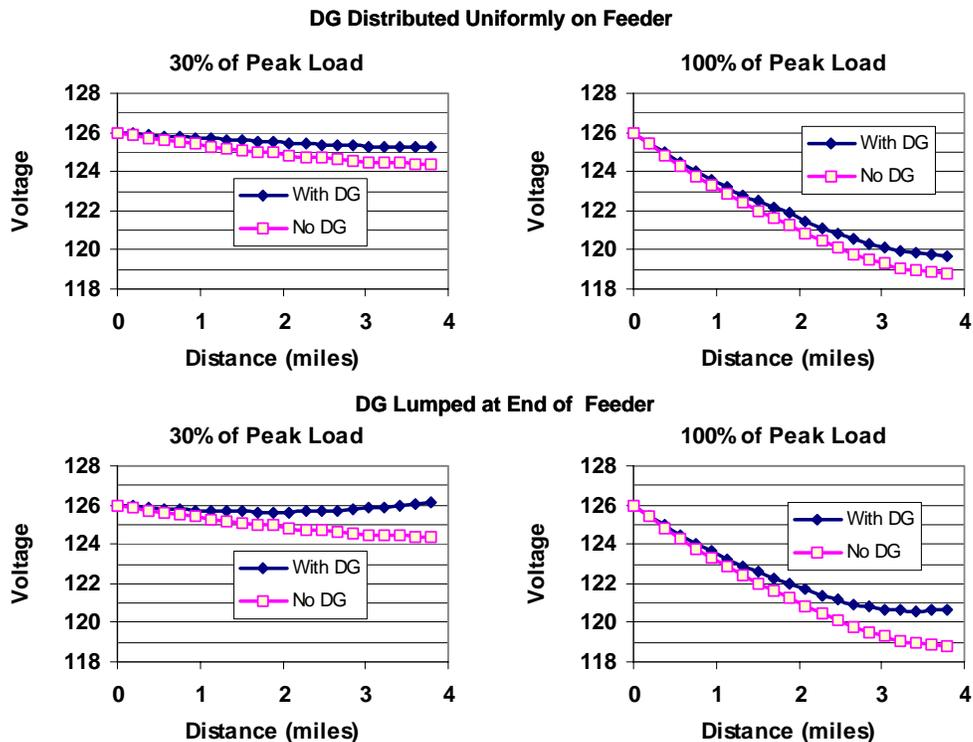
**Figure 4-5: Voltage profiles in a typical feeder with 30% DG penetration.**
