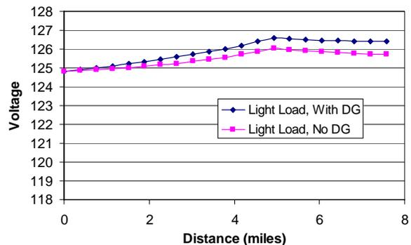
**Figure 4-6: Elevation of feeder voltage outside of ANSI C84.1 Range A; 20% DG penetration distributed over feeder. Fixed capacitor bank located at 5 mi.**
