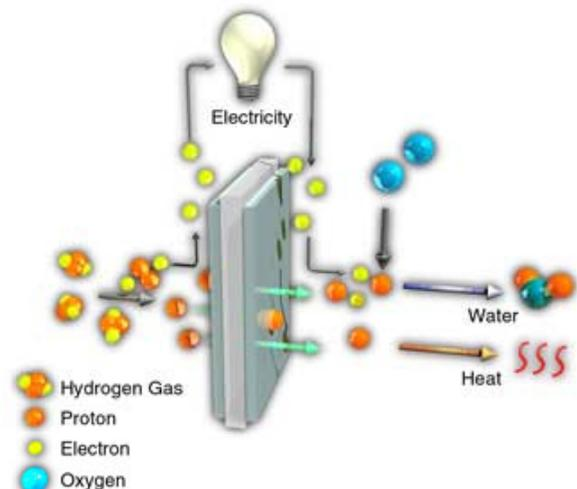
**Figure 3-3: Conversion of hydrogen and oxygen to electricity, water, and heat in a fuel cell**
