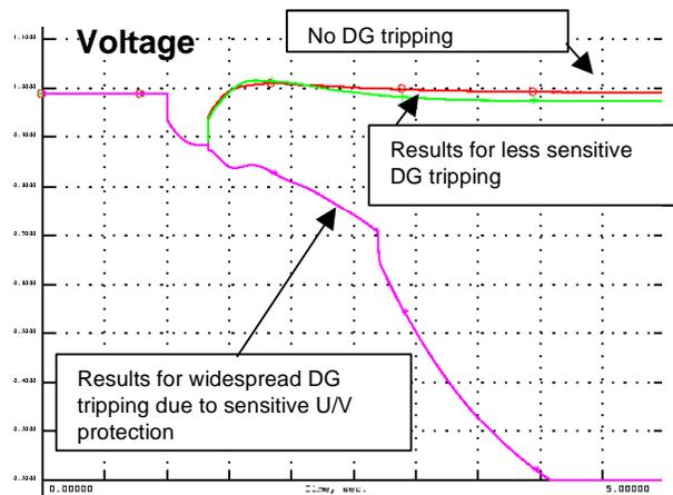
**Figure 5-1: Simulation of post-fault dynamic voltage behavior in a distribution system with DG capacity equal to 45% of load. Comparison of DG trip sensitivities.**
