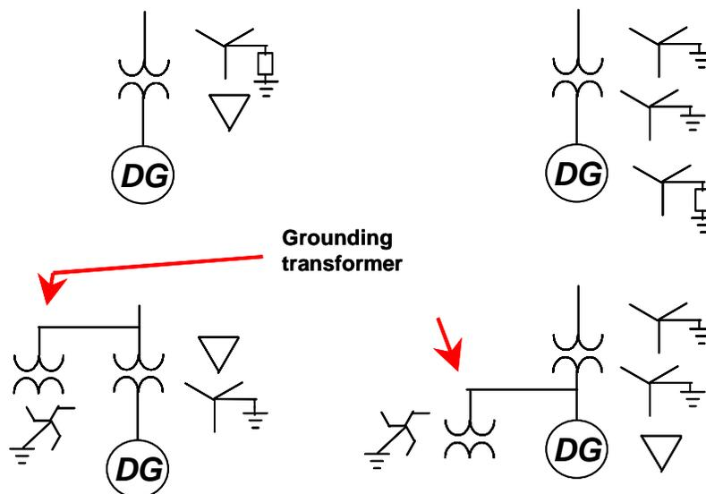
**Figure 4-4: Acceptable distribution transformer connections to provide primary grounding**
