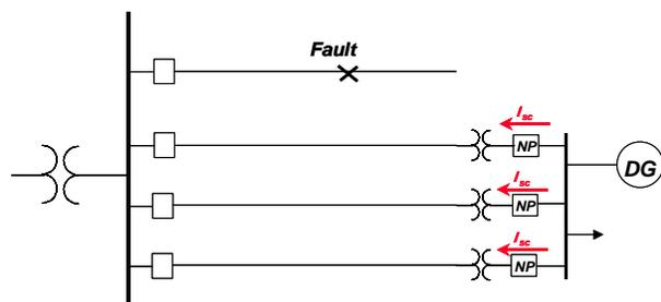
**Figure 4-13: Simultaneous reverse power flow through all the spot network's protectors due to DG contribution to an adjacent feeder fault**
