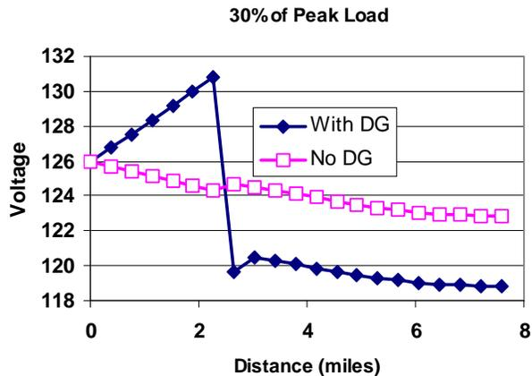
**Figure 4-9: DG voltage regulator and feeder SVR attempting to regulate same point to different voltages. DG penetration 100% of peak feeder load.**
