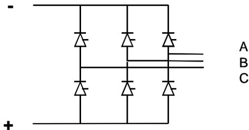
**Figure 3-11: 6-pulse load-commutated inverter bridge**
