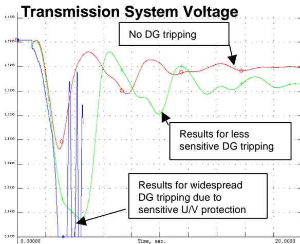
**Figure 5-2: Simulation of a transmission disturbance aggravated by DG trip sensitivity. System instability occurs for the most sensitive tripping.**
