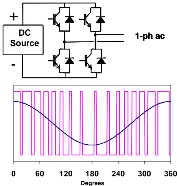
**Figure 3-13: Single phase VSI and generated voltage. Sinusoid is fundamental frequency component of pulse-width-modulated pattern.**
