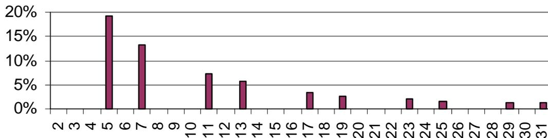
Figure 4-11: Harmonic currents produced by a typical 6-pulse load-commutated inverter.
