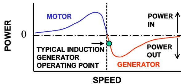
**Figure 3-10: Power-speed characteristic for a typical induction machine**
