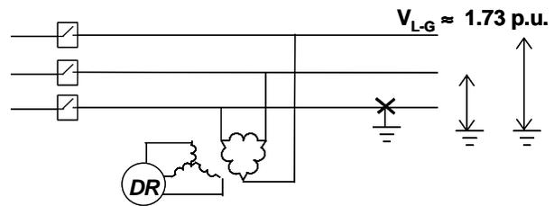
**Figure 4-3: Illustration of elevated primary phase voltage due to loss of grounding in island fed by DG**
