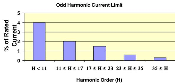
**Figure 4-12: Harmonic currents limits proposed for P1547. Even harmonics are limited to 25% of odd harmonic values shown above. Total rated distortion (root-sum-square of all components) is limited to 5%.**
